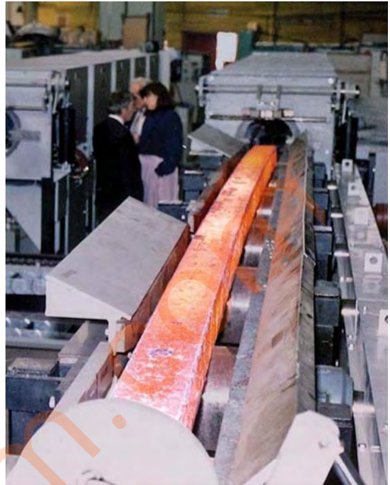
Figure 4. Dual-frequency induction heating of 4-inch x 4-inch x 10-foot bars has proved successful.
