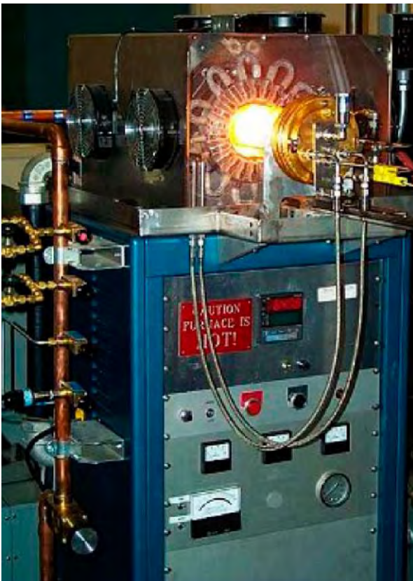
High vacuum, infrared system at ORNL
