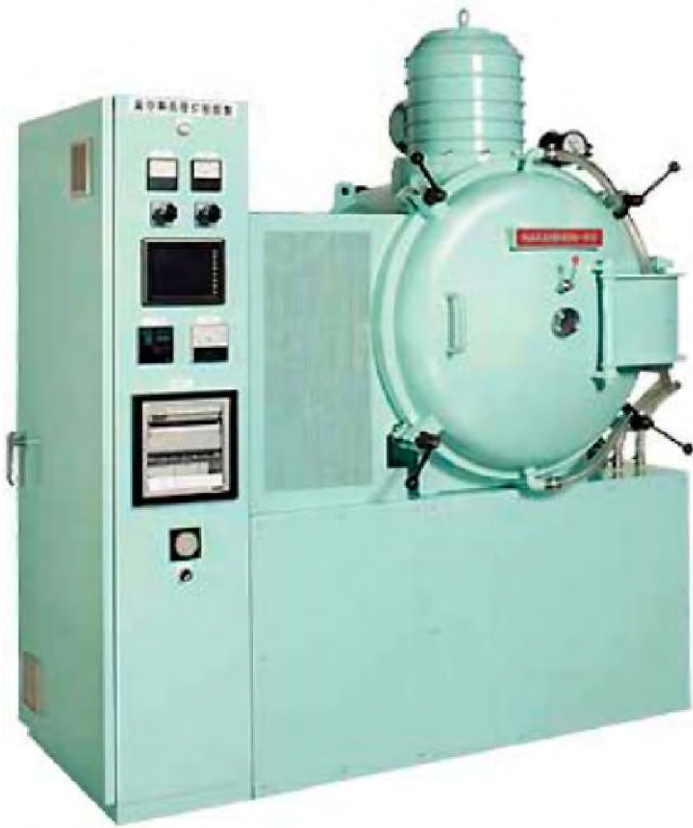
Typical small brazing vacuum furnace. From Nakanihon-Ro Kogyo.
